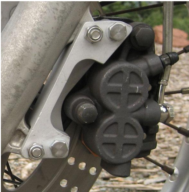
Done... I don't like the makers marks on bolt heads so I removed them. The new pads are EBC HH
