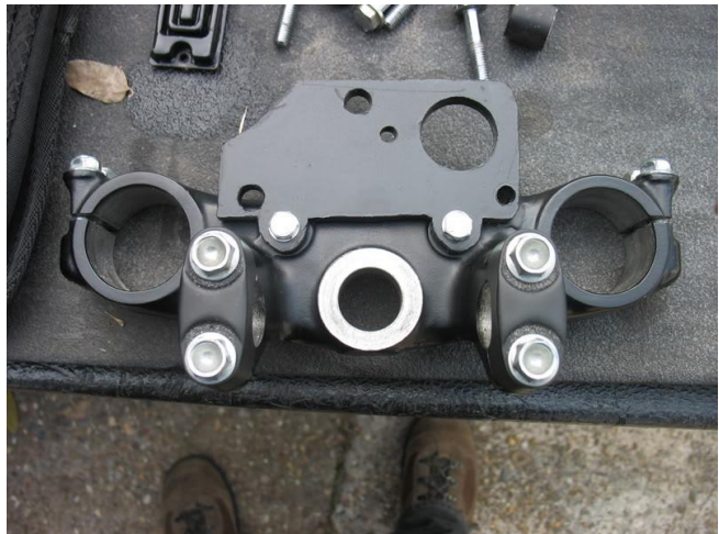
A pic of the modified upper clamp with the Keyswitch and Fusebox bracket installed.
