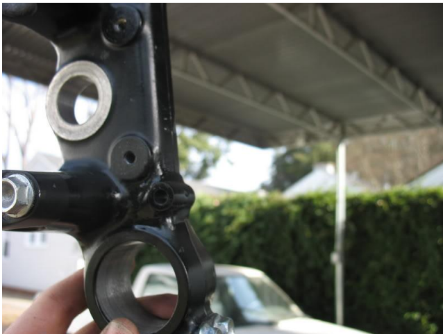
A pic of the modified upper clamp with the Keyswitch and Fusebox bracket installed.
