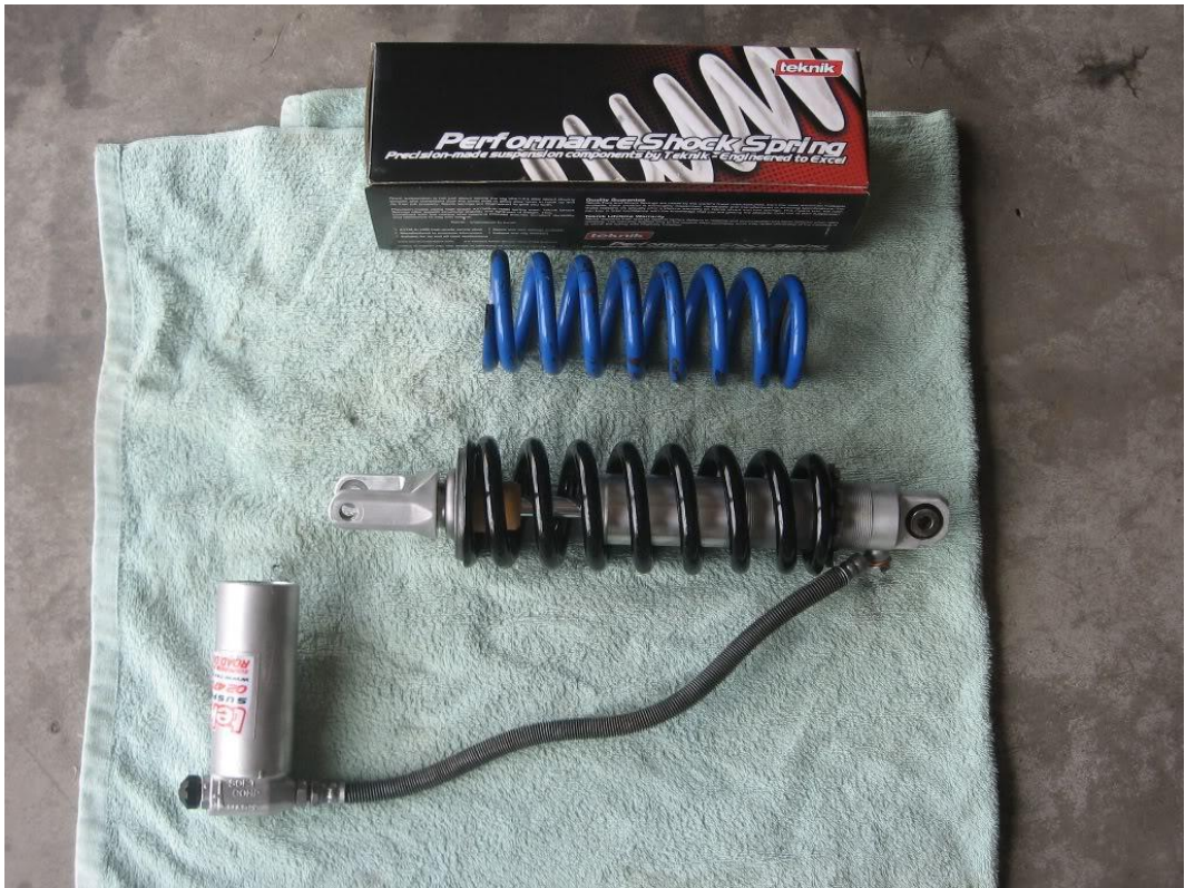
Above: Rebuilt shock. Note: original blue XR250R spring. Teknik could not supply a new rebound dial. I have one coming from Yamaha of Troy in the States.
